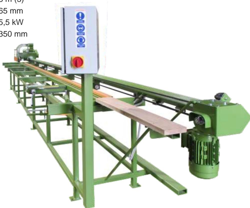
*The cutter is equipped with two gears that allow for longitudinal cutting of boards up to 20 and up to 36 cm wide. The use of movable splitting wedges means that the cutter can perform cuts in both directions.*
