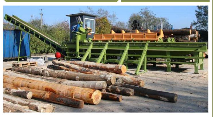
Purchase of a barker is a profitable investment that is frequently omitted in the sawmill sector. The use of barker for initial processing of wood allows for more effective selection of material, lower processing costs and protection of tools. It is also worth stressing that barking can form an additional source of income or fuel.
